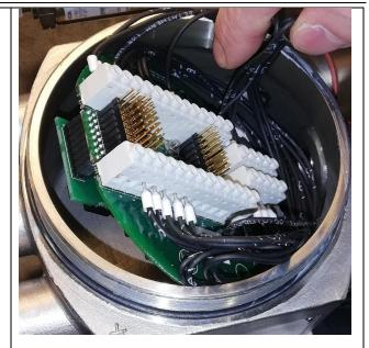
Move one wire at the time from the old PCB to the new PCB, starting from terminal 1 towards terminal 6
