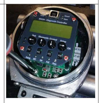
Gently remove the top PCB and expose the bottom PCB with the terminals
