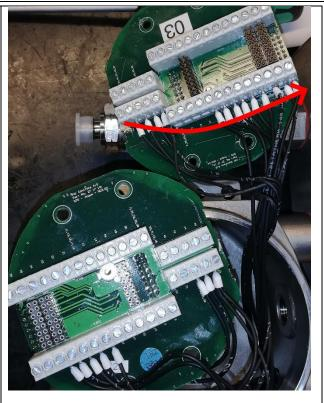
7 Gently position the new PCB in the Ex D enclosure by tilting it
