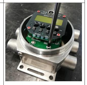
Remove the top PCB and gently disconnect the ribbon cable connecting the PCBs
